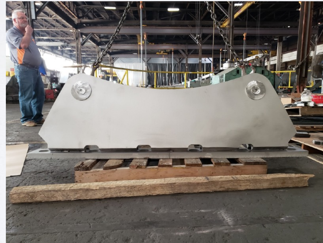
Base plates - splice joints - curved beams with splice joints and tapers
